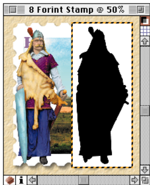
An image floater has two components; the RGB image and the visibility mask.
